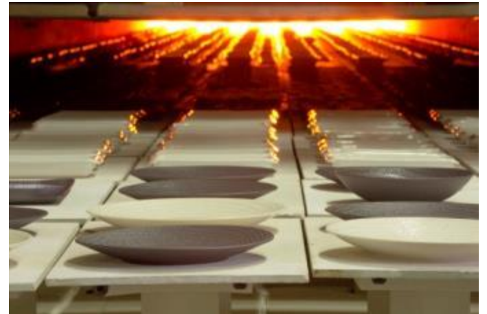
New tunnel oven of 45 metre (2014)
