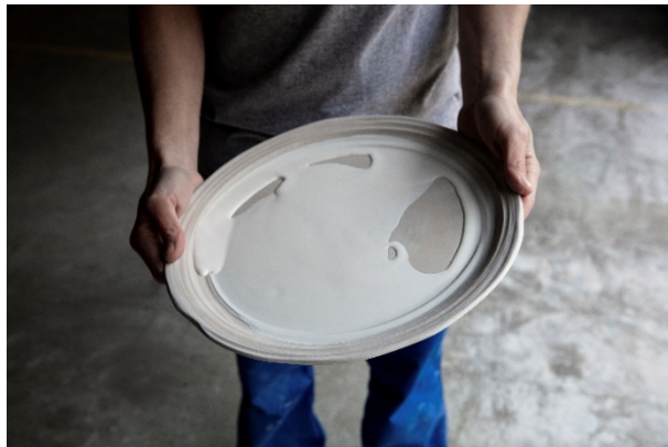
Recycled enamel is spread in the plate in the right quantity to assure a random rendering.
